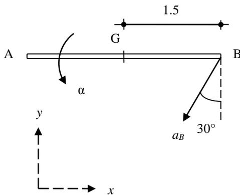
$$\begin{aligned} \overline{a_G} &= \overline{a_{G/B}} + \overline{a_B} \\ \overline{a_G} &= \overline{\alpha} \times \overline{r_{G/B}} + \overline{a_B} \\ \overline{a_G} &= \alpha k \times (-1.5i) - 0.5a_B i - 0.5\sqrt{3} a_B j \\ \overline{a_G} &= 1.5\alpha j - 0.5a_B i - 0.5\sqrt{3} a_B j \end{aligned}$$
